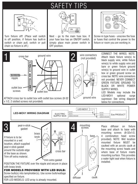
CAUTION: Do not turn on without diffuser installed. Do not touch LEDs or circuit board. LED optics could be damaged. No lamp replacement required! Integral LED light engine supplied. Do not remove protective cover from LED light engine.
