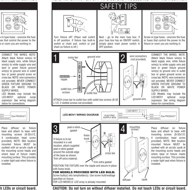
CAUTION: Do not turn on without diffuser installed. Do not touch LEDs or circuit board. LED optics could be damaged. No lamp replacement required! Integral LED light engine supplied. Do not remove protective cover from LED light engine.
