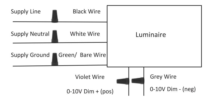
For dimming wires, use class 1 wiring methods. Cap dimming wires (separately) if not used.
