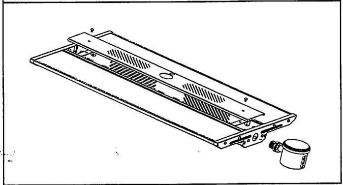
3. Open the junction box cover to the position shown in the figure (half open state), move away the knock-out, the microwave sensor go through the knock-out, fix the gasket, screw and tighten it.
