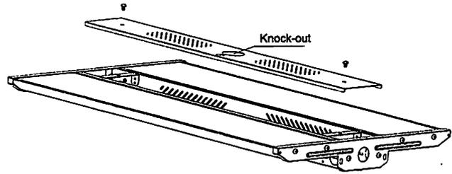
3. Open the junction box cover to the position shown in the figure (half open state), move away the knock-out, the microwave sensor go through the knock-out, fix the gasket, screw and tighten it.
