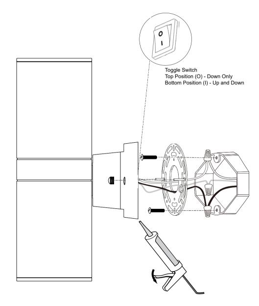
Apply silicon around luminaire perimeter after installtion
